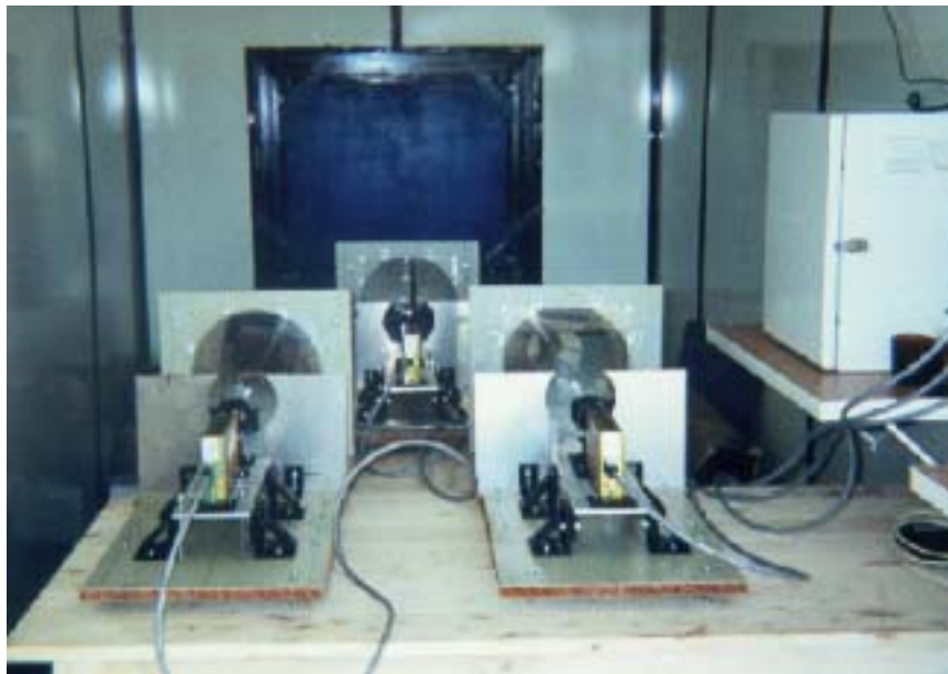
Fig. 1. Three light sources are shown facing the UV transmitting window. The white enclosure (on shelf) contains the solar power regulator and storage battery.
