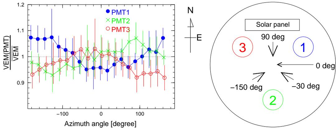
**Fig. 2.** Ratio of the signal of each PMT to the average of 3 PMTs as a function of azimuth angle of the air shower. Primary cosmic ray zenith angle smaller than 60 degrees and 10 or more  $\overline{VEM}$  are required. In this plot, a clear azimuthal effect is evident.
