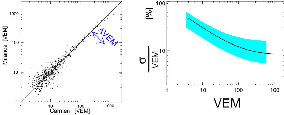
**Fig. 1.** Left: Correlation of the signals recorded in Carmen and Miranda. The distance of each point to the solid line is the fluctuation of each particular event. Right: Signal fluctuation between Carmen and Miranda as a function of the average of the two signals. The shaded area shows the uncertainty due to event selection. The solid line is representative of the data on average and indicates a fit using Equation (1) resulting in  $A = 0.08$  and  $B = 0.80$ .
